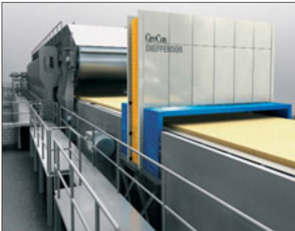
DIEFFENSOR: protects press steel belts and optimises the spreading quality
