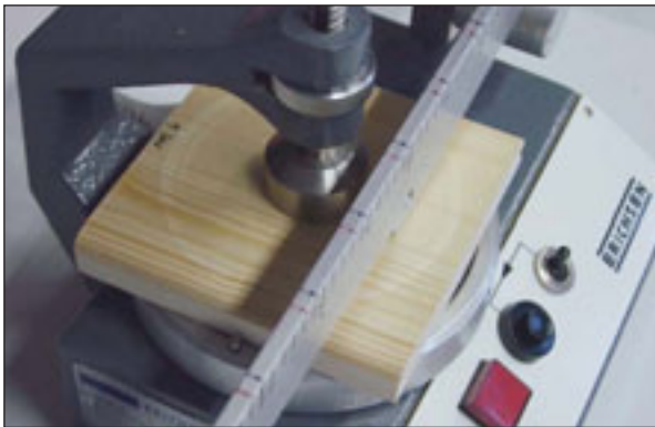
b) The scratch test according to EN438-2.14
