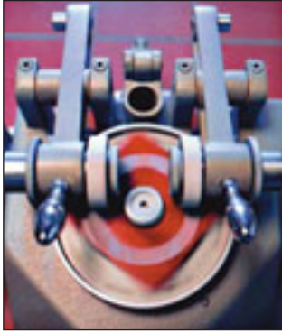
a) The taber test according to EN438-2.6 and EN13329
